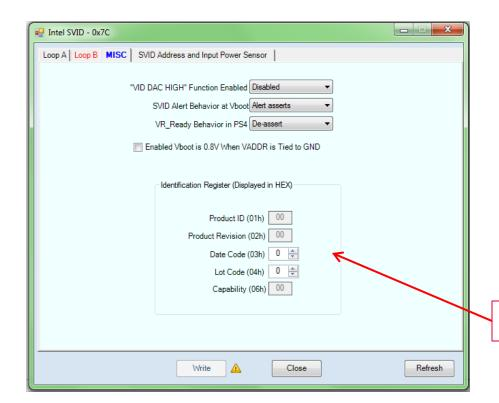
Readout of identification data stored in Voltage regulator
