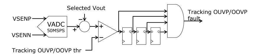
4 consecutive samples over/under the limit will trigger the fault.
