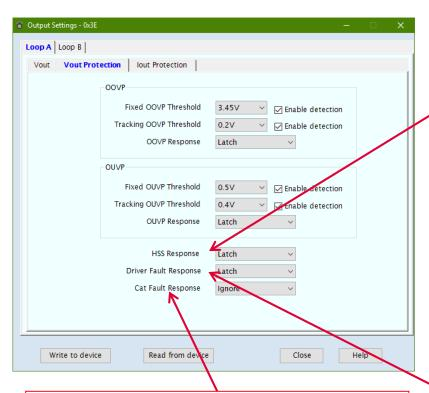
**Cat Fault Response:** What to do if a Catastrophic fault is detected.
