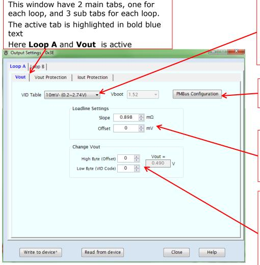
**VID table** allow selection of VID voltage step. Here the part is in AMD mode and only one selection possible. Therefore it is grayed out and not changable
