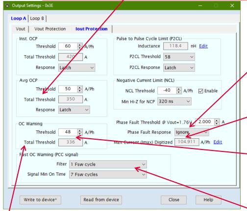
**Total threshold** is calculated from the Threshold entered and the GUI knows number of phases to present the total output current where the warning trigger.
