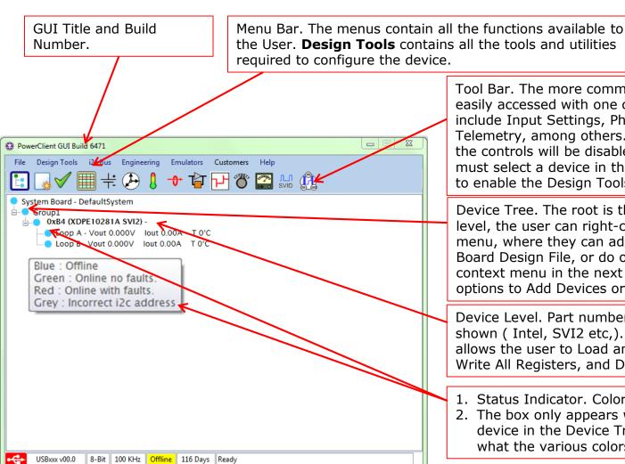
Tool Bar. The more commonly used Design Tools can be easily accessed with one click on these icons. These include Input Settings, Phase and Frequency, and Telemetry, among others. When a device is not selected the controls will be disabled and gray colored. The user must select a device in the Device Tree by clicking on it to enable the Design Tools.
