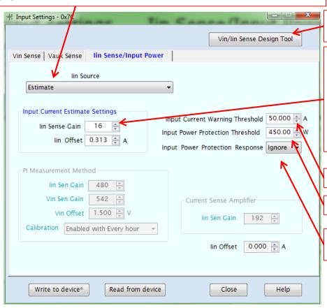
Opens a new window for the **Input Sense Design Tool** that help calculate settings
