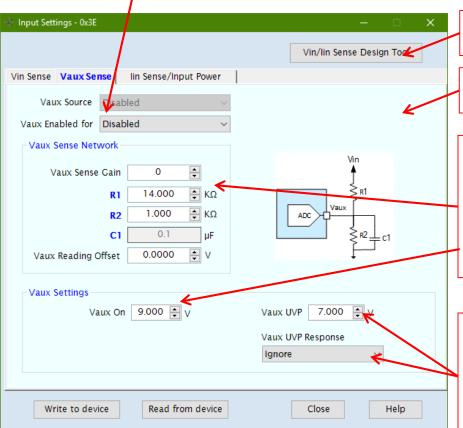
Opens a new window for the **Input Sense Design Tool** that help calculate settings
