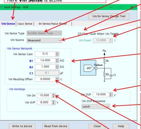
Clear Fault When Vin Toggle: If checked the fault flag will clear itself when Vin is removed and then restored
