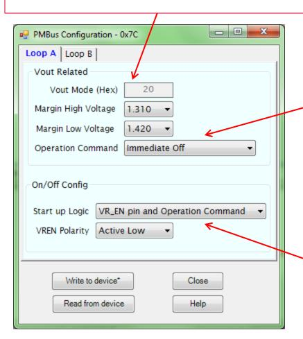
Selection of Margin voltages ( if used) and the configuration of the Operation command.
