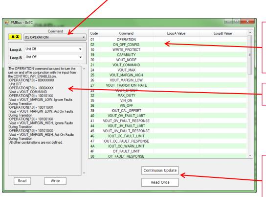
List of each PMBus command and if a controller is connected it will read out the settings and list them in easy to read formats.
