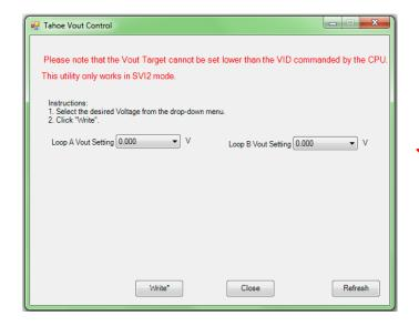
This opens a window that allow manual selection of output voltage.
