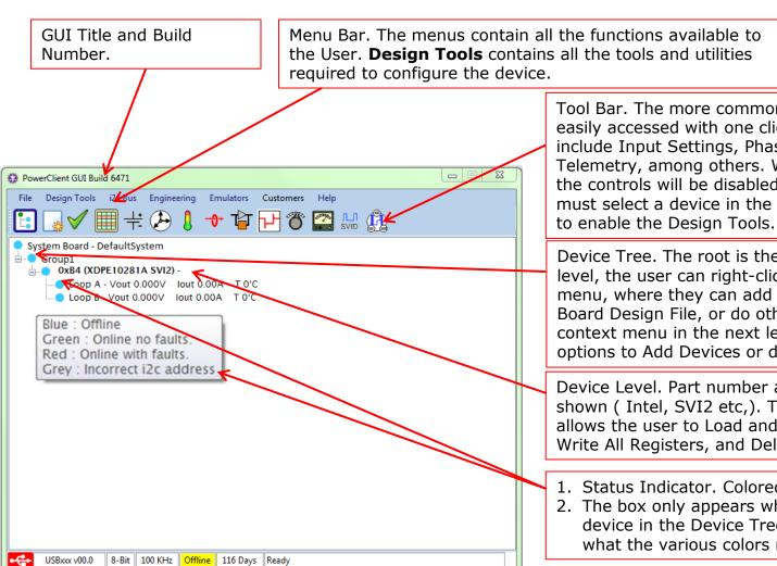
Tool Bar. The more commonly used Design Tools can be easily accessed with one click on these icons. These include Input Settings, Phase and Frequency, and Telemetry, among others. When a device is not selected the controls will be disabled and gray colored. The user must select a device in the Device Tree by clicking on it
