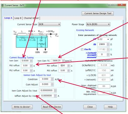
**Isen Gain TC** (Temperature Coefficient) This setting value is between 2000  $\sim$  4000 ppm/degC typically. Use the ideal copper TC=3906.25 first and then based on temperature compensation result of inductor DCR to trim this value. This value could be different by layout.
