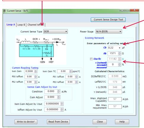
**Power stage.** When Current sense Type is selected to be Non-DCR then the family of powerstage used can be selected here. In this example grayed out and not selectable as DCRsense is selected.
