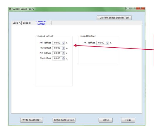
**Ph1 (Phase1) loffset**. Additional offset for reported value. Behavior does depend on if current sharing is active or not. When no current sharing each phase get the individual offset. When current sharing active then any offset entered is shared equal between all active phases even of offset is only entered for one phase.
