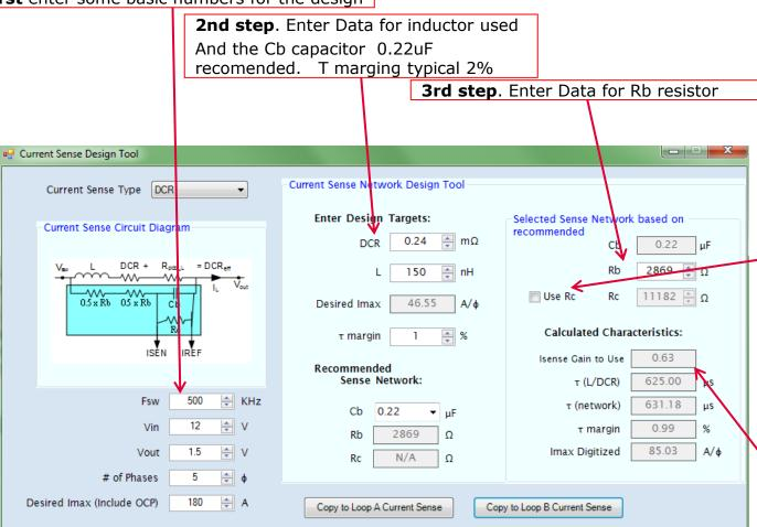
Use Rc. If there is a high DCR value the sense voltage may be needed to be divided down by using resistor Rc. If this is used mark the box and enter a number in the Rc field
