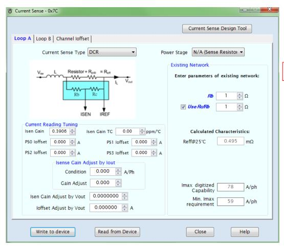
With a sense resistor instead of DCR sense most settings are similar.
