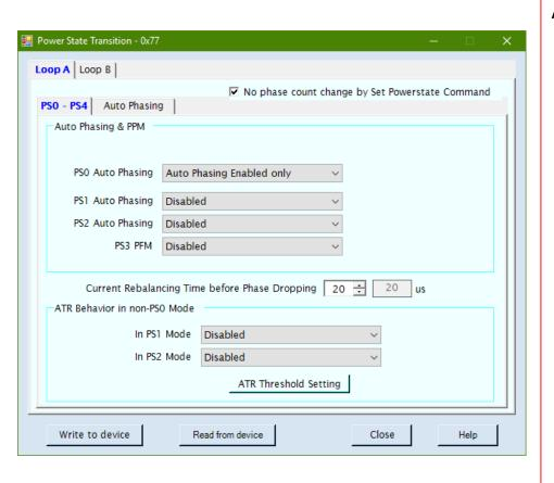
Auto Power State Definitions PS0→ more than 1 phase operation oIOUT is greater than the 'phase add' current threshold PS1→ 1 phase (or 2 phase) operation oIOUT is less than 'phase add' current threshold oIOUT is greater than PS2 threshold PS2→ Diode Emulation, Constant ontime, variable frequency oIOUT is less than PS2 threshold (typically set between 5A and ½ inductor ripple current) PS3 oSame as PS2 For AMD PS0=normal operation PS1=PSI0 L PS2=PSI1 L
