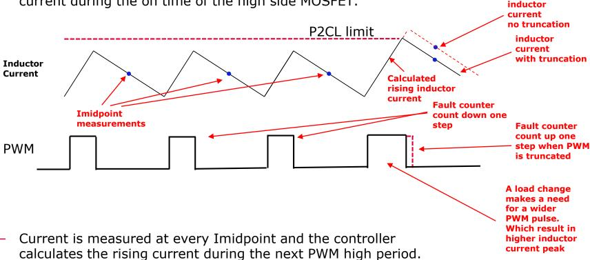
When the calculated current reaches the P2CL limit the PWM will be truncated
