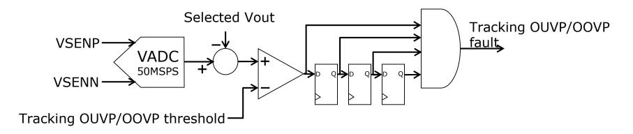
4 consecutive samples over/under the limit will trigger the fault.
