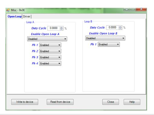
In open loop mode, output voltage faults (OUVP) protection and all ATR events must be disabled to prevent premature shutdown and false tripping of the ATR.
