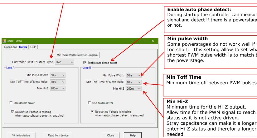
During startup the controller can measure each PWM signal and detect if there is a powerstage connected
