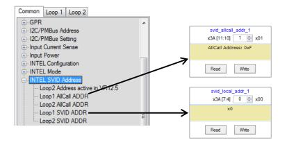
In Common Section under INTEL SVID Address
