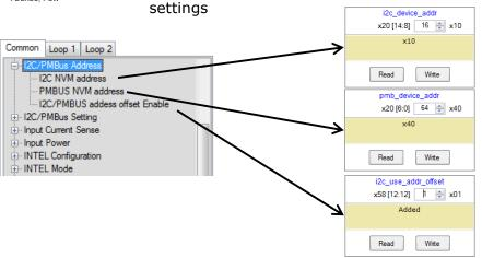
In Common Section under **I2C/PMBus Address** I2C and PMBus device address can be programmed accordingly. An external i2c address offset resistor can also be enabled(1) or disabled(0).
