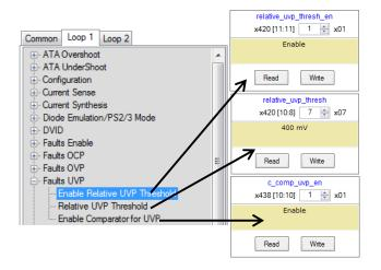
In Loop 1/Loop 2 section under Faults UVP
