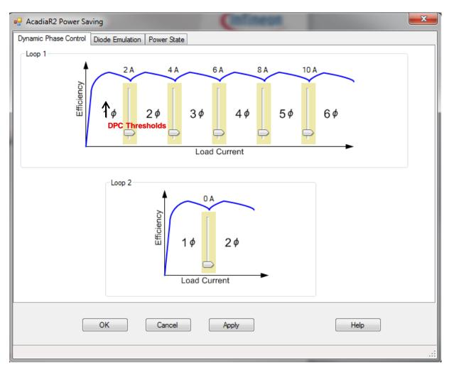
The **Dynamic Phase Control (DPC)** allows users to configure the VR to autonomously and dynamically add or shed phases as the load current varies to optimize efficiency over a wide range of loads. The **DPC thresholds** set the output current level at which a phase is added. **Note:** This can be set to 0A to not use DPC.
