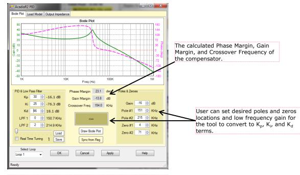
The compensator follows this transfer function, ωρ, and ωp<sub>2</sub> are configurable poles to filter noise and roll of the high frequency gain that the K<sub>d</sub> term creates.
